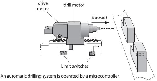
Part of the control program includes a sub-procedure 'Drill' which will activate when a component is detected on the conveyor belt.
